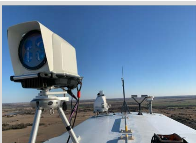
Lidars and a disdrometer were installed on the top of a nacelle of a wind turbine in the King Plains wind farm as part of the AWAKEN project. Nacelle-mounted instruments provide valuable observations of the local flow and atmosphere at hub height that have a powerful influence on wind turbine energy production and response. Photo by Andy Scholbrock, NREL
