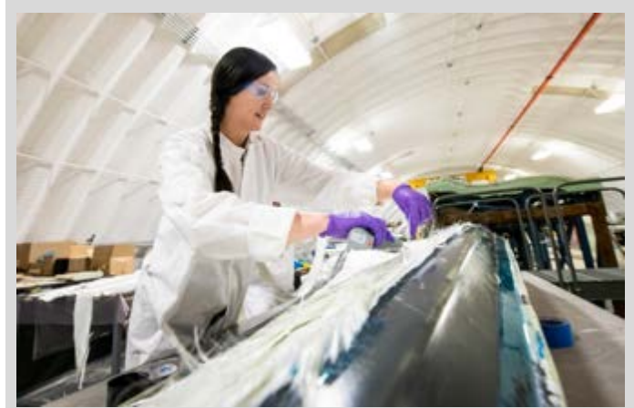
An NREL study evaluated the benefits and limitations to 3D-printed wind turbine blades, which are traditionally hand built, like this blade at NREL's Flatirons Campus. Photo by Dennis Schroeder, NREL
