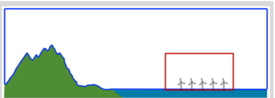
This illustration shows how the ERF model will work with the AMR-Wind model to simulate an offshore wind farm adjacent to non-flat terrain. Graphic by Bruce Perry, NREL
