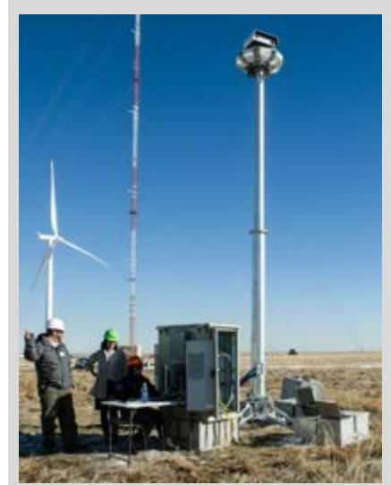
Identiflight reduces interactions between raptors and wind turbines by using cameras to curtail selective wind turbines when raptors approach. Photo by Dennis Shroeder, NREL
